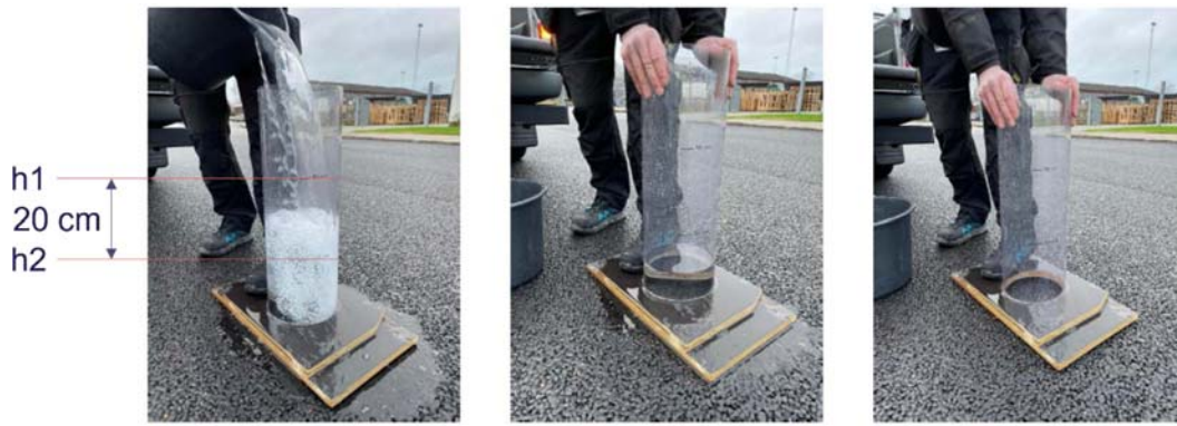
Fig. 2. Beckers Method Test Arrangement on Field (Water is filled up until h1 and the time is measured until h2)
