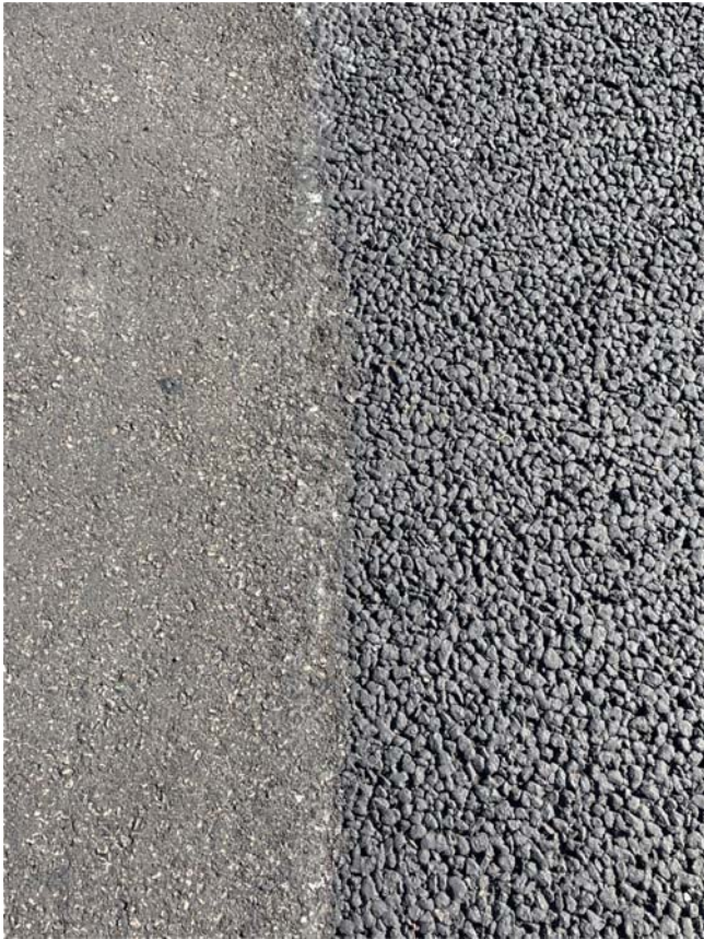
Fig. 1. Left Image Shows a Surface of Traditional Asphalt, and Right Image Shows Porous Drainage Asphalt
